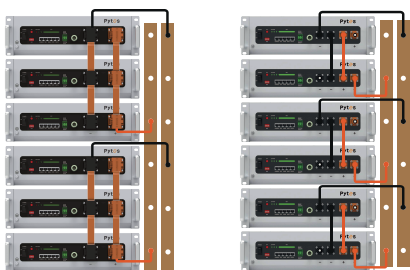
Figure 5-1 Schematic diagram of power cable connection
